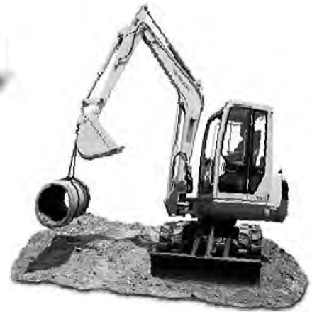
TB145 10,494 lbs Height 8'5" Width 6' Bucket Sizes - 24" Hammer - 750 lbs
