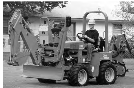
RIDE-ON TRENCHER W/ BACKHOE ATTACHMENT 3700 - 6"x 48"
