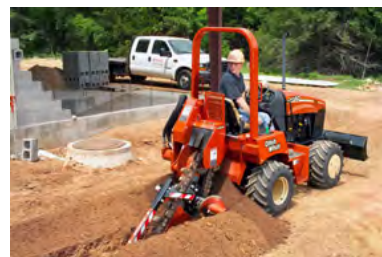
RIDE-ON TRENCHER W/ BACKHOE ATTACHMENT 3700 - 6"x 48"
