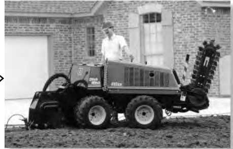
410 SX PLOW 18" DEPTH TRENCHES 3' DEEP
