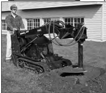
TX 420 COMPACT UTILITY TRAC LOADER WITH AUGER Bits Available 6", 12", 18", 30" WHEELED & TRACK
