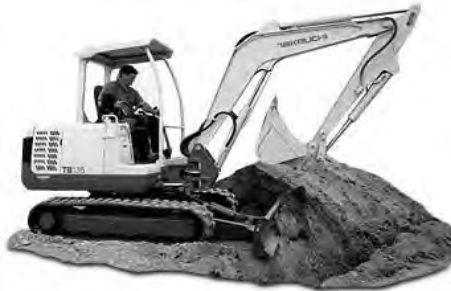
TB135 7,606 lbs Height 8' Width 5'4" Bucket Sizes - 12", 18", 24" Hammer - 750 lbs
