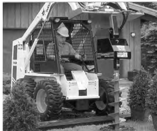
POST HOLE AUGER BOBCAT SERIES 24 MOUNT Bits Available 6", 8", 12", 16", 24"
